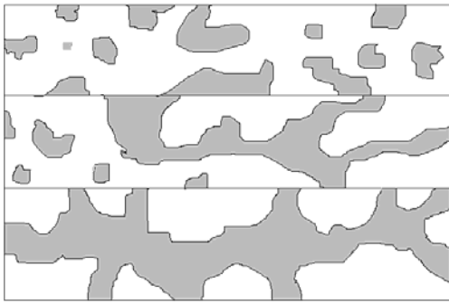
Fig. 2 - Scheme of infinite cluster formation from conducting particles in anisotropic polymer matrix
