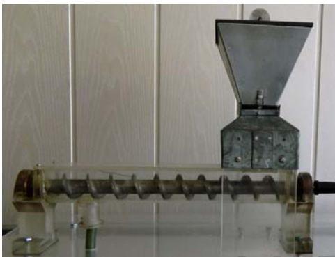
Figure 6 – The metering screw conveyer batcher of a dust
