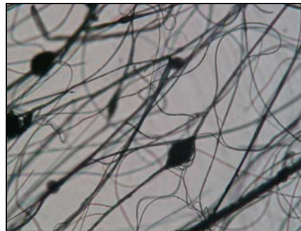
Fig. 1 □ Optical microscope micrograph of 16% PANi blend solution, beads can be observed clearly.
