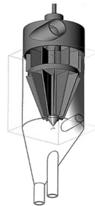
Fig. 3 - Geometrical model of a scrubber
